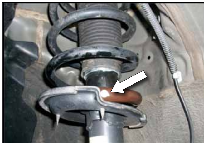
Shown in photo: Installed protective cover on lower spring loop.
