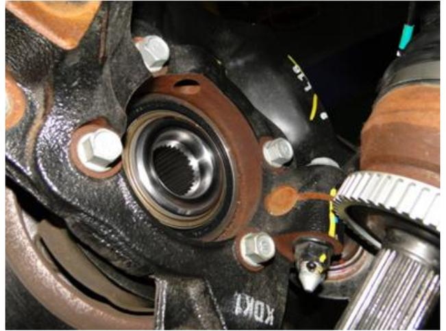
9. Install the replacement drive shaft washer (I).
